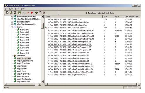
*N-TRON*®'s IndustrialSNMP (iSNMP) Suite software specifically designed for the industrial marketplace, provides monitoring and analysis of *N-TRON*'s 600, 700, 7000, and 9000 Series Industrial Ethernet Switches, as well as other SNMP capable Switches. iSNMP suite provides a real- time view of the health of your Ethernet network devices, the overall network traffic volume and status from within an HMI software environment.
