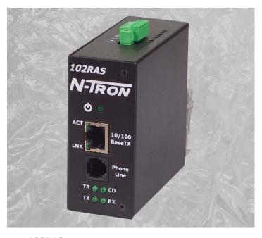
The 102RAS server supports three security options. The "fixed" callback option stores a password and the remote user's phone number. Once the remote site enters their password, the 102RAS calls back using the number stored in its database. The "variable" option lets the user, such as road warriors, enter a fixed password and a variable call back number each time they call. The "pass through" option offers the security of password protection, while bypassing the call back process.
