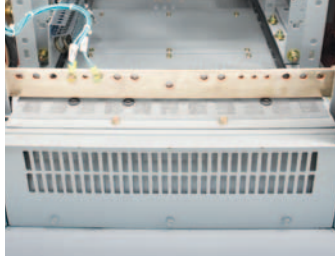
Rear Bottom Vent w/Dynamic Flap
